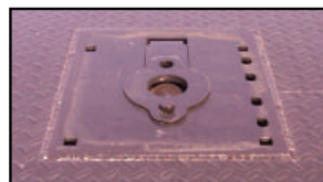
Retractable ball hitch for quick hook ups.
