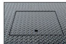
Gooseneck style hinged door, flush mounted. 8" structural channel drawbar included.
