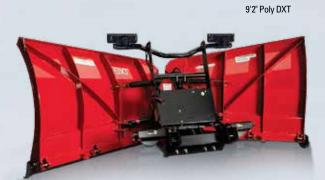
Patented Dual-Trip Design combines Trip-Edge and Full Moldboard Trip technologies on every DXT plow for protection from obstacles in any position, high or low.
